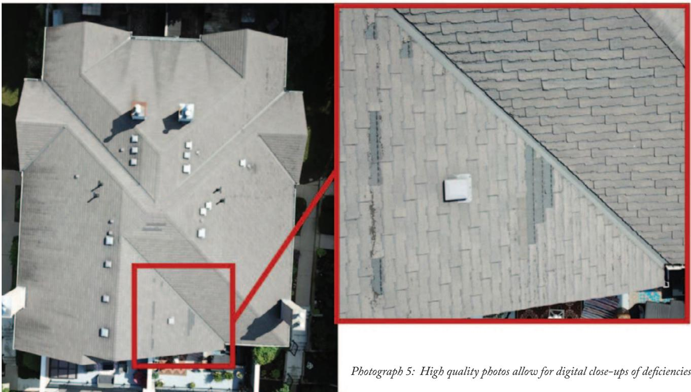
*Photograph 5: High quality photos allow for digital close-ups of deficiencies.*
