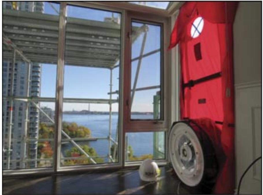
*Figure 2 – Air leakage testing in progress at condominium building in Toronto. The blower door (red) is used to either pressurize or de-pressurize the building interior. Photo credit: RDH Building Science Inc.*
