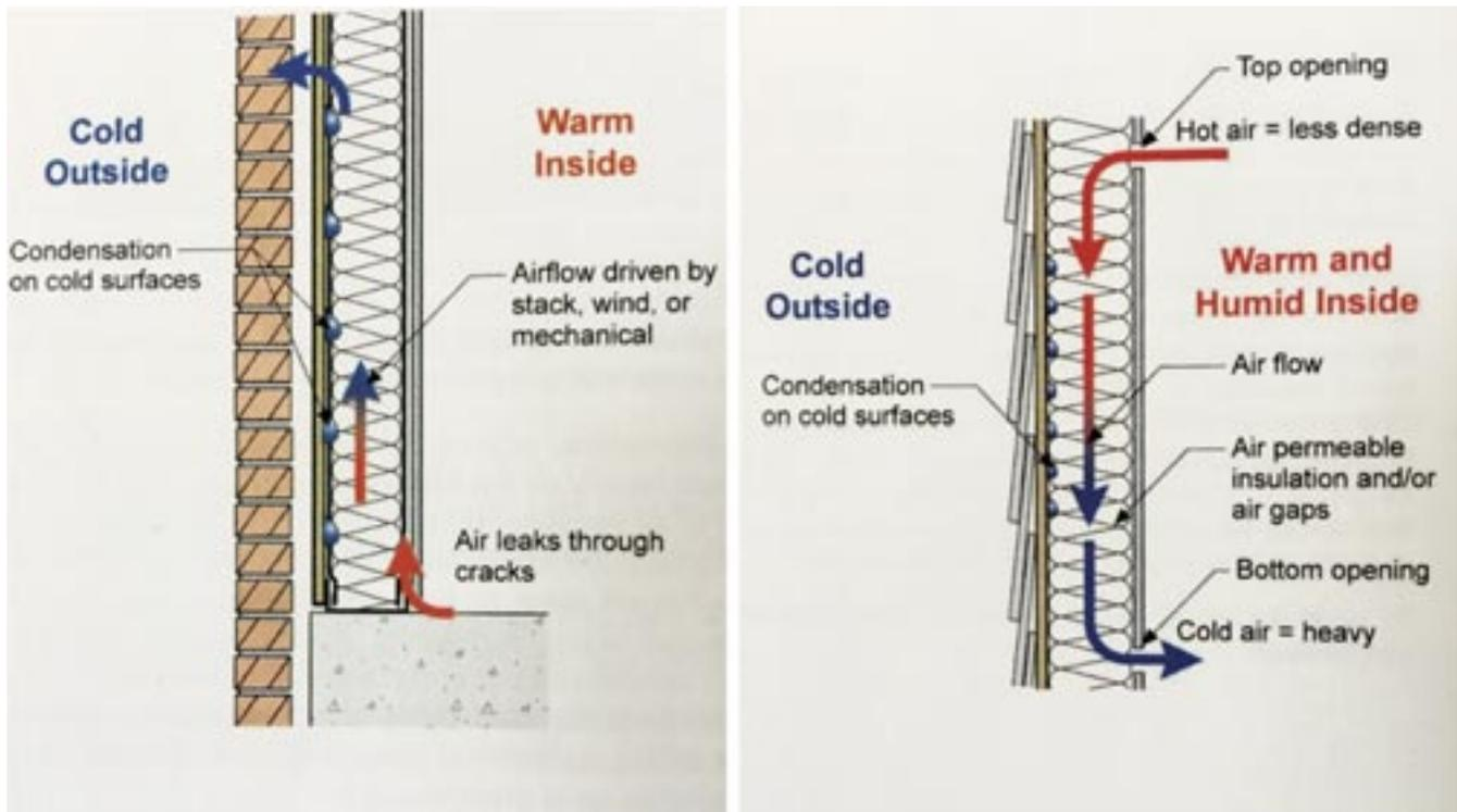
Figure 1 – Two ways in which condensation can form in an exterior wall. Both cases are caused by warm air contacting the cold exterior sheathing. Image credit: High Performance Building Enclosures. © John Straube and Building Science Corporation.
